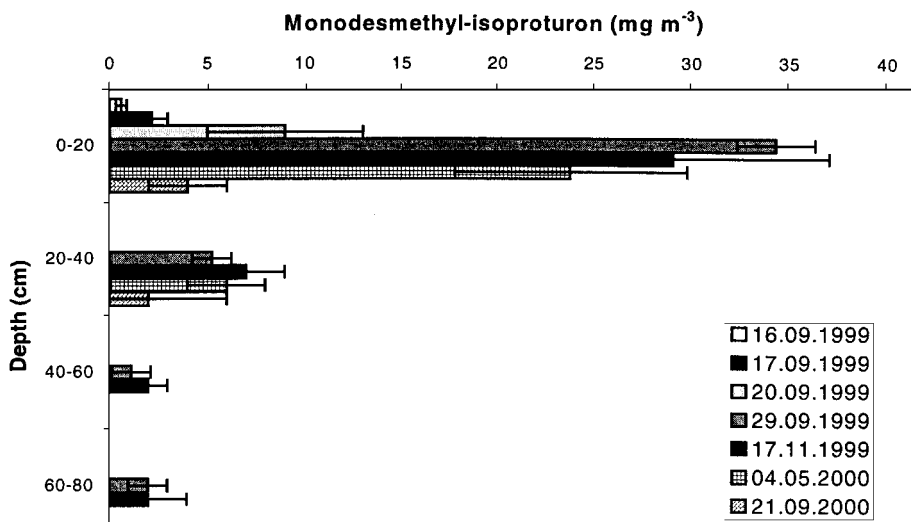
FIGURE 9 Concentration and distribution of the major metabolite monodesmethyl-isoproturon (MMU) ( \text{mg m}^{-3} ) as measured at the experimental field from 16.09.00 to 21.09.00 ( n=3 ).
